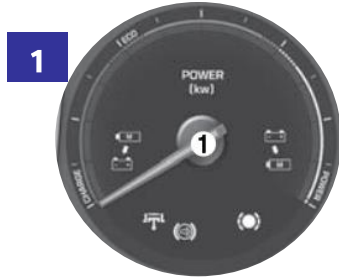
1 : Regeneration brake/ECO/power gauge
